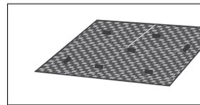
EN - Use 2x30cm anchors/m<sup>2</sup> on slopes >2:1. Use 1x20cm anchors/m<sup>2</sup> on flat surfaces. Or use pins.
